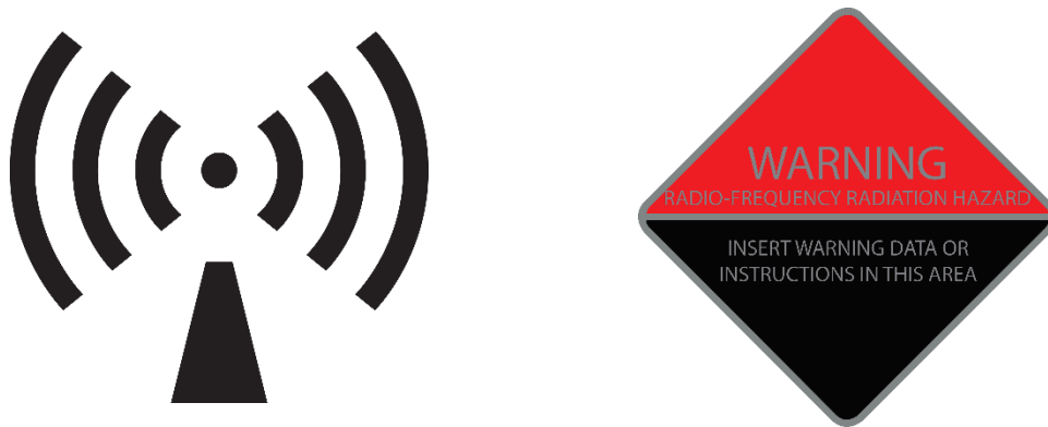
Figure 9. The OSHA RF energy advisory symbol and the California radio frequency radiation warning sign. The lettering for the California warning sign must be legible at a distance of 10 m (i.e. the letters must be at least 75 mm high).
