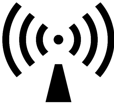
Figure 9. The OSHA RF energy advisory symbol and the California radio frequency radiation warning sign. The lettering for the California warning sign must be legible at a distance of 10 m (i.e. the letters must be at least 75 mm high).
