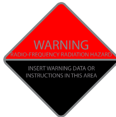
Figure 9. The OSHA RF energy advisory symbol and the California radio frequency radiation warning sign. The lettering for the California warning sign must be legible at a distance of 10 m (i.e. the letters must be at least 75 mm high).
