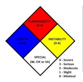
NFPA 704 is part of the Accident Prevention Warning Signs that are placed on the door or wall prior to entering an area where the hazards may be present. They are intended to provide emergency responders with the information they need to determine the immediate actions to be taken in an emergency.
